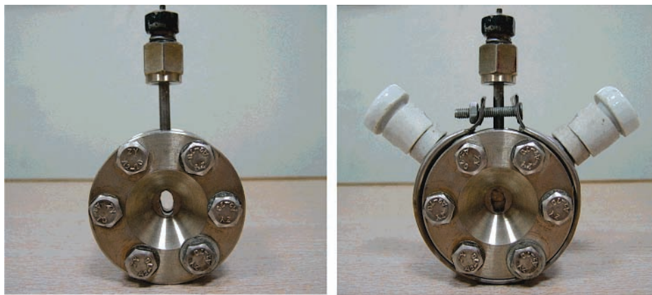
Figure 1. Synthesis cell for in situ XAS (left) and that with Be windows and heating component mounted (right).
